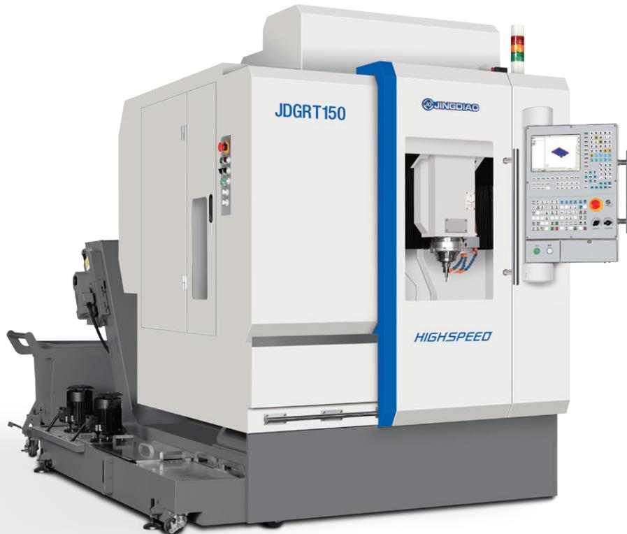
Adopting the full closed-loop control technology, suitable for 5-axis machining of precision parts and complex hardware.
